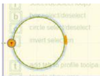
Figure 5 ♦ Adding tabs to profile toolpaths means that the work won't become loose, and is held securely throughout the machining operation
