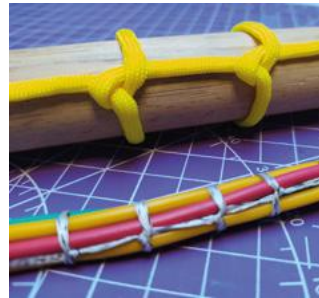
Figure 11 □ An example of the running lock stitch with the last one on the right tied incorrectly with a common error
