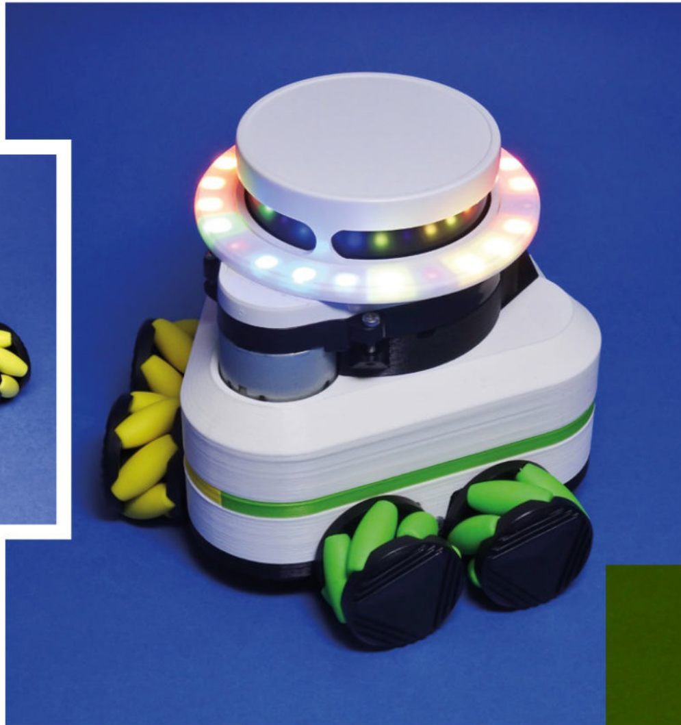
Above ↗ L-Hex in all its RGB, Mecanum-wheeled, lidar-using glory
