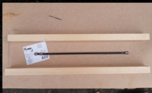
Left ♦ MDF isn't the most pleasant material to work with; it blunts tools, it looks dull, and it kicks up a load of toxic dust when you cut it with power tools. The advantage it has is that it doesn't warp, and it's relatively cheap
