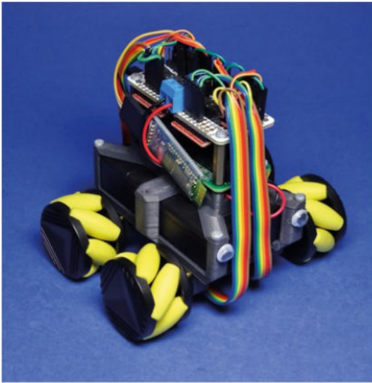
Above ↗ The Mini Mecanum robot showing its stack of components
