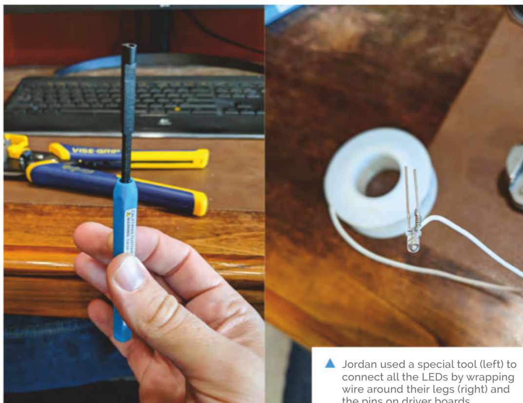
▼ And so it begins... wire-wrapping connections to a couple of LEDs on one of the eight PWM driver boards – only 189 more to go!
