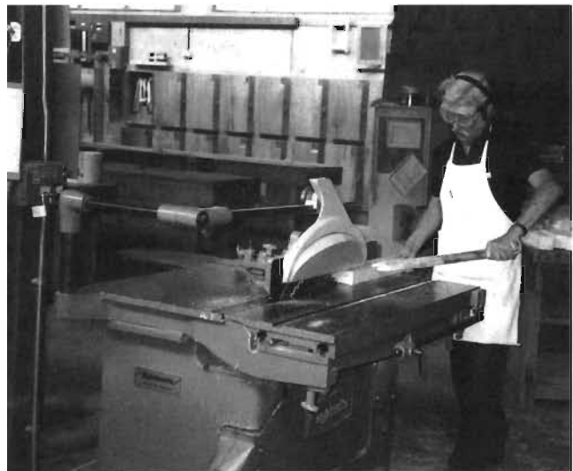
Figure 7.2 Using the dimension saw. Note the safety precautions (goggles, ear protection, guard in use).
