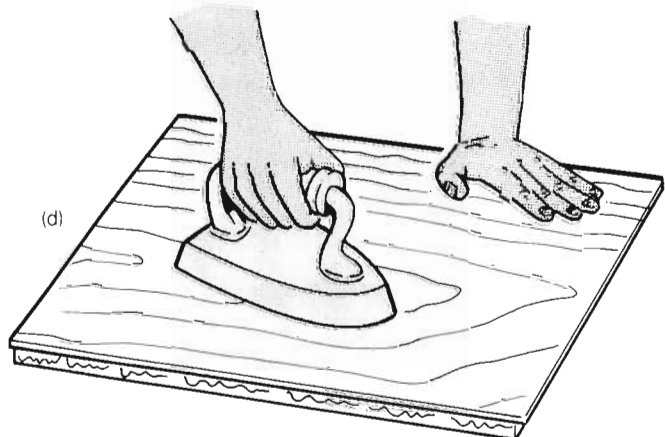
Figure 10.4 Hammer veneering: (a) cutting veneer, (b) preparing the ground, (c) squeezing out surplus glue, (d) Melting chilled glue.
