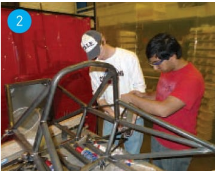
2. Belter and Jaju test-fit the uprights on the welded chassis.
