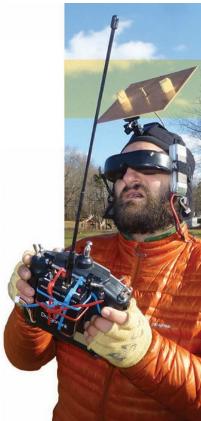
Georgi Tushev's head-mounted FPV ground station sports a large flat high-gain "patch" antenna.
