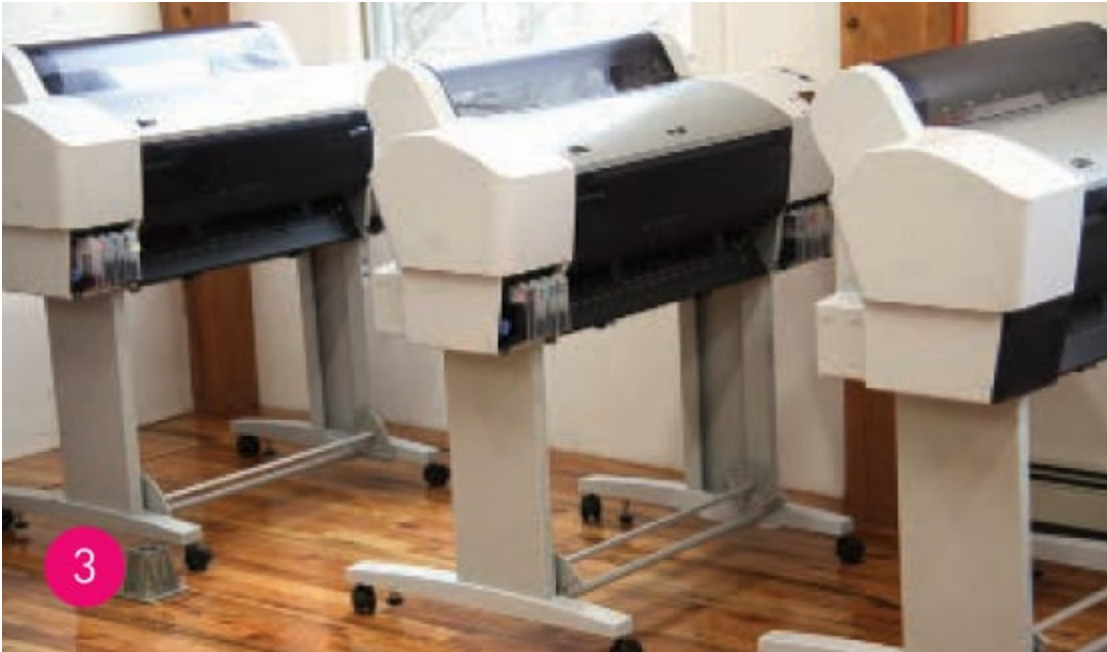
3. Three Epson 7880 printers — each has been converted to Cone's Piezography inks using refillable cartridges. Each printer has a different "color" of black and white inks. One is Carbon, another is Selenium, and the third is Neutral.
