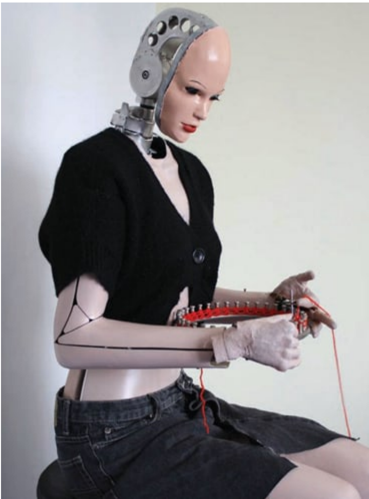
Agnes’ arms contain electric motors salvaged from old desktop printers.
