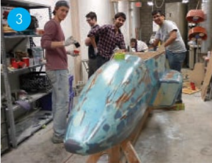
3. The plug gets a final release coat before being used to make the fiberglass molds, which are then used to create the carbon fiber body.
