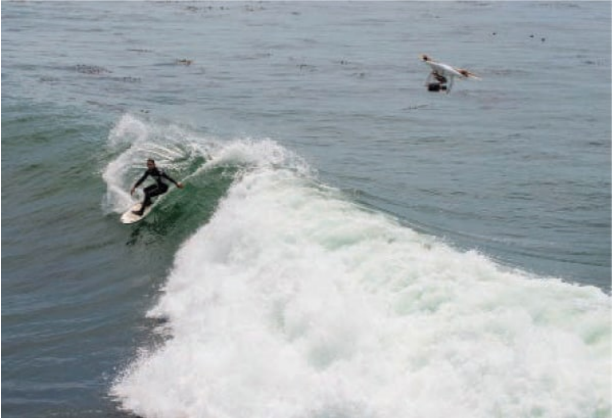
The aircraft is crooked but the camera is level, controlled by a brushless gimbal. Eric Cheng
