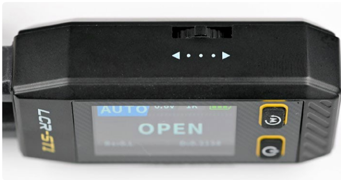
Figure 3: The three-way switch on the side allows selecting most settings of the device.
