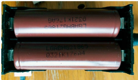
▲ Figure 5: The two 18650 Li-Po housed in the battery holder. Due to the high average current values, it's advisable to head to the PCB version of those cells (with tabs), and solder them directly to the PCB.
