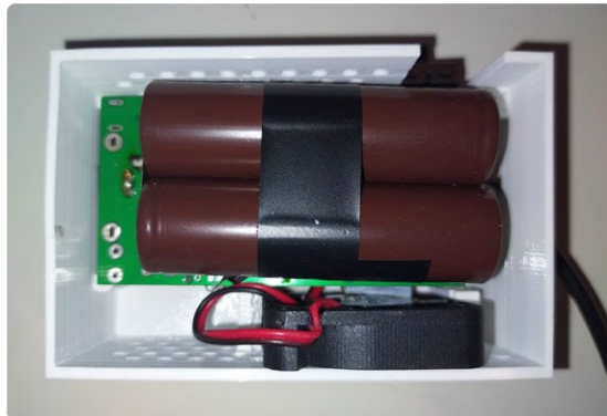
▶ Figure 7: The small fan has enough space in the housing, tailored on purpose.
