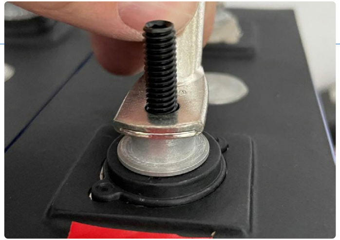
Figure 10: Close-up showing the terminal posts (Source: Martin Jepkens).
