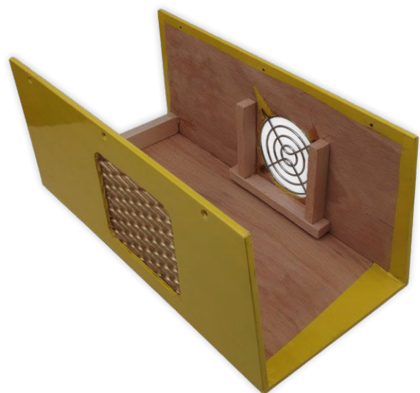
Figure 9: The round opening corresponds to the diameter of the intake side of the fan. The bars ensure that almost all the air drawn in is from outside.
