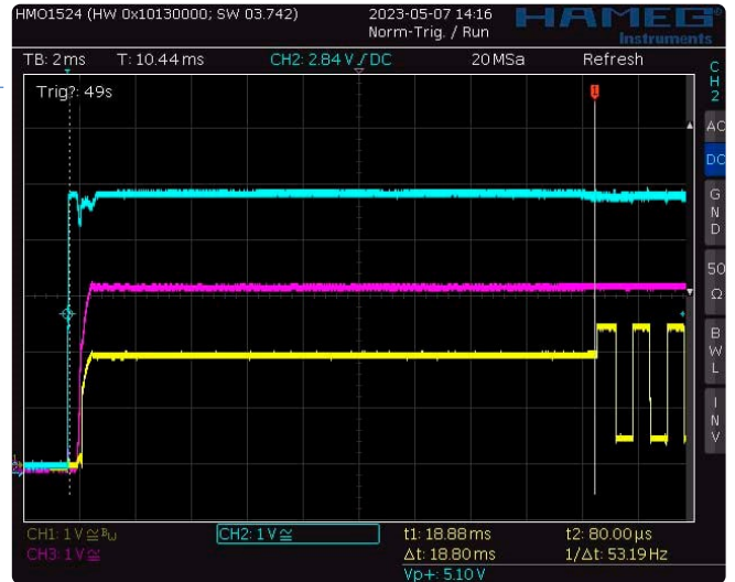
Figure 3: Switch-on process of the Raspberry Pi Pico.
