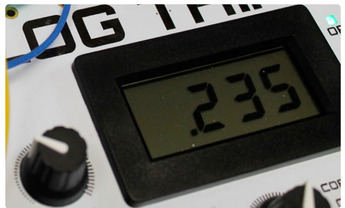
Figure 2: The panel meter is for setting coefficient values, not for displaying signals produced by the analog program.
