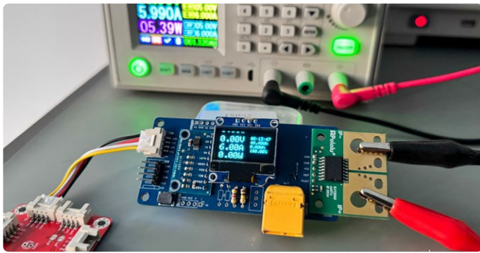
Figure 6: The AmpVolt v2.0A in action demonstrating current measurement during testing.
