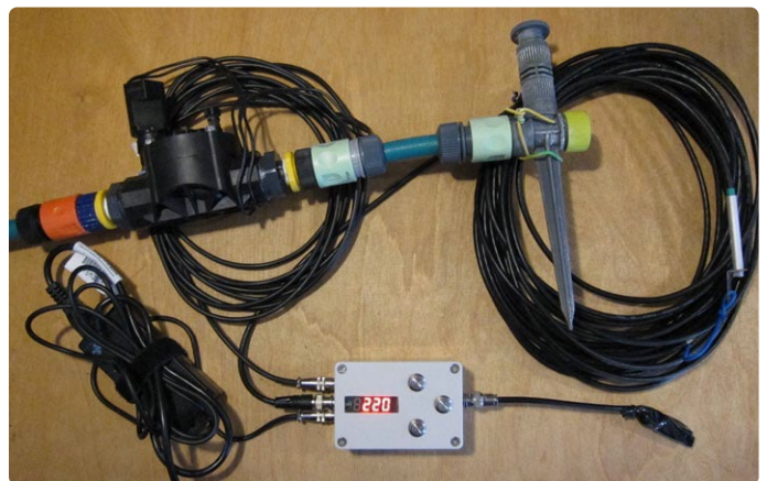
Figure 1: All the components of the frost guard system.
